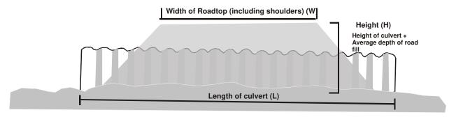
Determining the length of a culvert:
